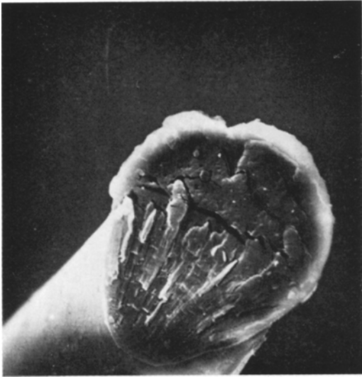
Figure 21 15 denier nylon 6 fibre (strain rate 8 \times 10^{-4} \text{ sec}^{-1} ) at breaking extension of 39% ( \times 680 ).
